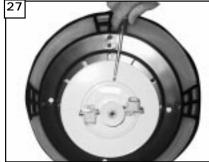
Use the 3 screws removed in step 21 to put fitter on to fan.
